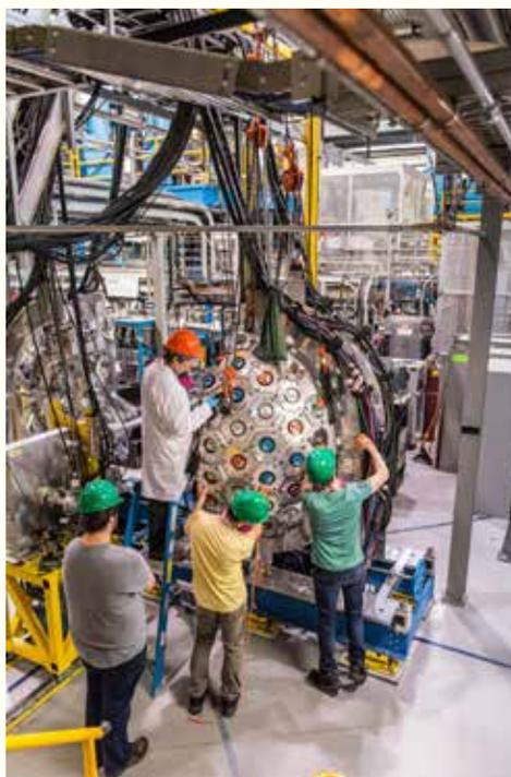
Researchers working on the DESCANT neutron detector array at TRIUMF.
