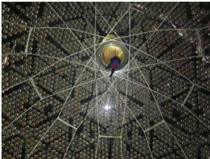
Scientist being lowered into the SNO+ acrylic vessel to prepare the detector for filling.
