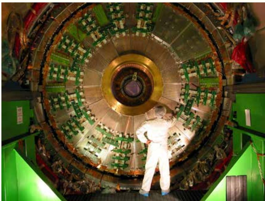
The Canadian built Hadronic Endcap Calorimeter for the ATLAS experiment at CERN.
