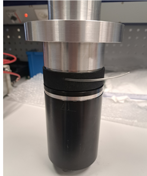
(d) The PMT base attached to the window assembly, with part of the clear ring used to connect them sticking out for demonstration.
