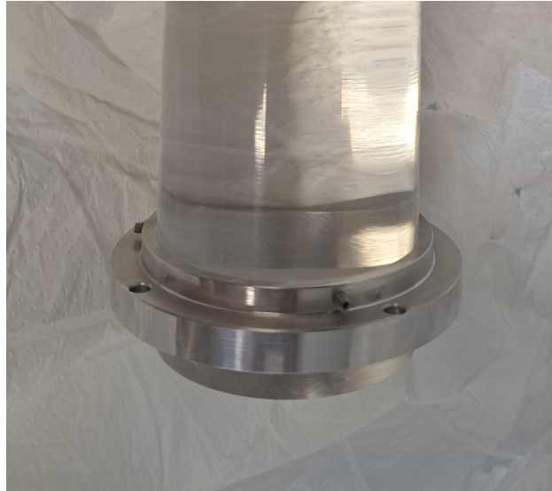
FIG. 8: The ring clamp on the bottom of the fishtail light guide.
