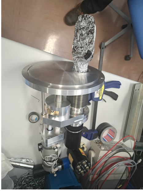
FIG. 10: The completed assembly, including the PMT and its base, the scintillator and light guides, and the motor and bellows.
