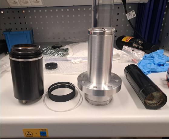
(a) From left to right: the PMT base, the screw ring to connect the PMT to the window assembly, the window assembly (with the light guide attached), and the PMT.
