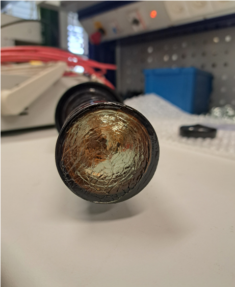
(c) The PMT photocathode with a layer of optical grease.
