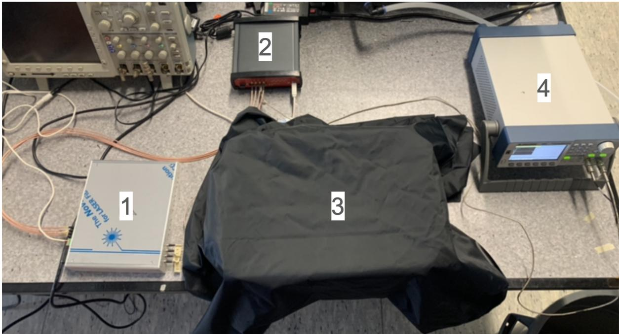
Figure 6: A photo of the SiPM testing setup used for room temperature characterization at TRIUMF.
