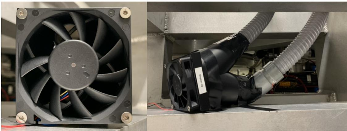
Figure 16: Images of the cooling fan attached to the Barrel Veto. The pipes lead to 2 separate ASD cards.
