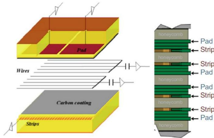
Figure 1.5: Components of a layer of an sTGC. The pad, the wires and the strips give the position of the measurement. [1]
