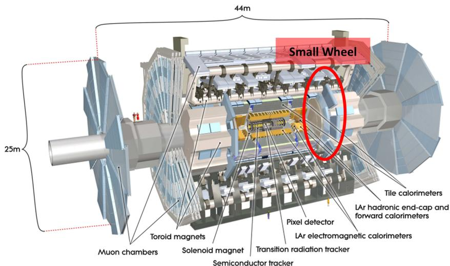
Figure 1.3: The ATLAS experimnt. The collision between beams of particles happens at the center of the detector and the created particles are detected by various instruments. The future emplacement of one of the NSW is shown in red. [5]
