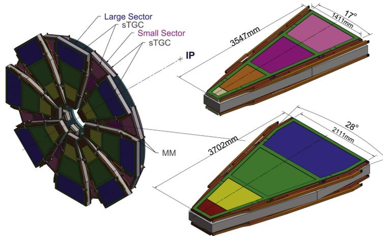
Figure 1.4: Schema of the New Small Wheel. sTGC are a technology used in this muon detector. [1]
