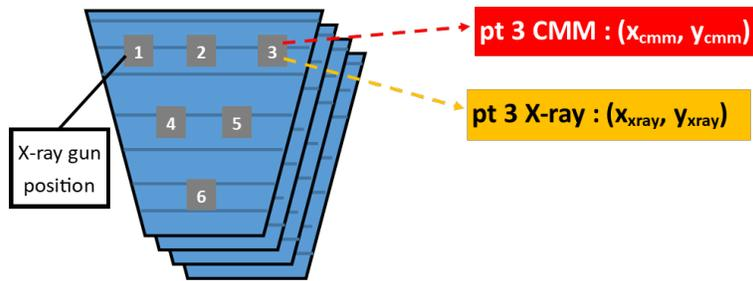
Figure 2.1: Schematic representation of x-ray gun positions along the surface of a quadruplet. For each x-ray points, there is a set of coordinates for CMM measurements  $(x_{cmm}, y_{cmm})$  and another for x-ray measurements  $(x_{xray}, y_{xray})$ .
