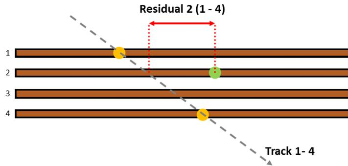
Figure 2.4: Definition of a track residual. The residual 2 (1-4) (in red) is the difference between the real position of the measurement in the layer 2 (in green) and the position obtained by taking into account the reconstruction of the track with fixed layer 1 and 4 (grey array).
