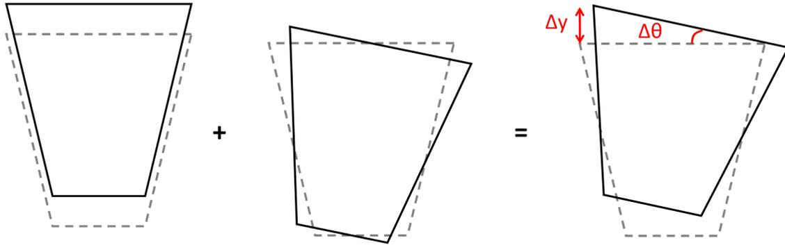
Figure 2.2: *The misalignments occurring during the quadruplets' construction considered in the analysis. For each layer, there is a definite offset and a definite slope.*
