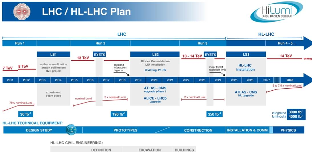
Figure 1.2: The High Luminosity LHC project planing. From 2011 to the end of the project, the energy of the particles would have been doubled and the luminosity multiplied by ten. The NSW will be installed during ATLAS experimnt Phase-1 upgrade (LS2). [2]
