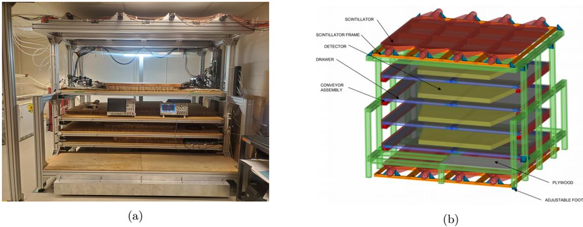
Figure 2.3: McGill cosmic ray test stand. (a) is the setup that detects muons at McGill [6] and (b) is a schematic of the cosmic-ray detector [7]
