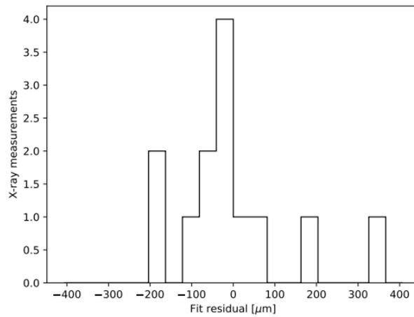
Figure 3.2: Histogram of the difference between  $y'_{cmm}$  and  $y_{xray}$  for the QL3P05 quadruplet's layer 4 x-ray points. As a result of the fit, the sum of these differences is minimal.
