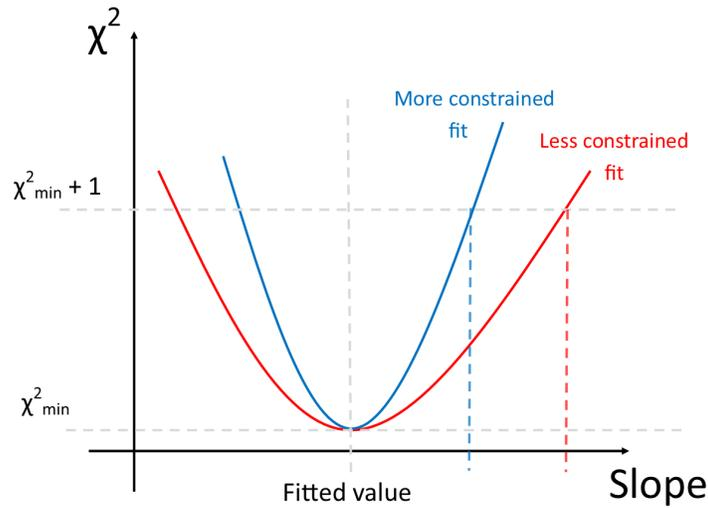
Figure 2.5: Representation of the minimum of a  $\chi^2$  function, related to the uncertainty on the value, as a function of the slope or the offset. Most of the time, adding a constraint to the minimization of the function leads to a narrower "parabola-like" function around the minimum, and so it gives a smaller uncertainty on the value.
