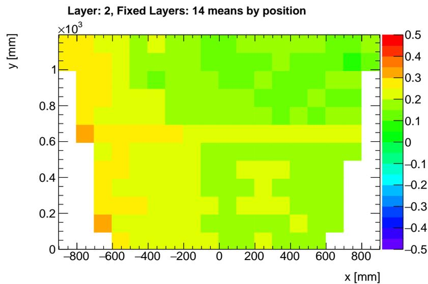
Figure 3.3: Track residuals 2 (1-4) of the QL2C04 quadruplet (3100V). For different point along the layer, the track residual is calculated. [6]
