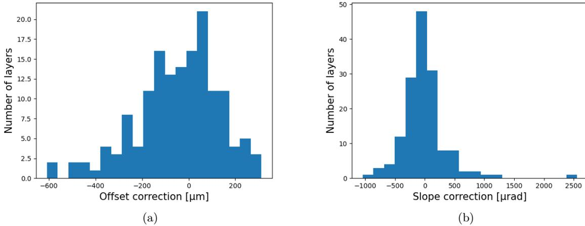
Figure 3.1: *Correction of the misalignments that occurred during the quadruplets' construction for 153 layers. Corrections of a few hundred micrometers and a few hundred microradians are respectively observed for the offset ((a)) and the slope ((b)).*
