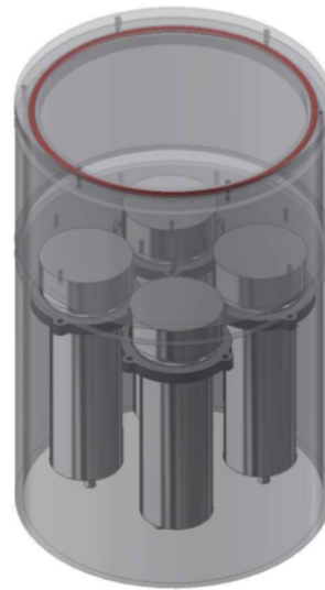
Figure 1: CAD drawing of SCOUT showing acrylic vessel atop four PMTs.
