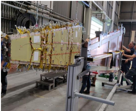
Figure 10. Sector assembly. Left: MM wedge, Right: sTGC wedge [Madhoun, 2019].
