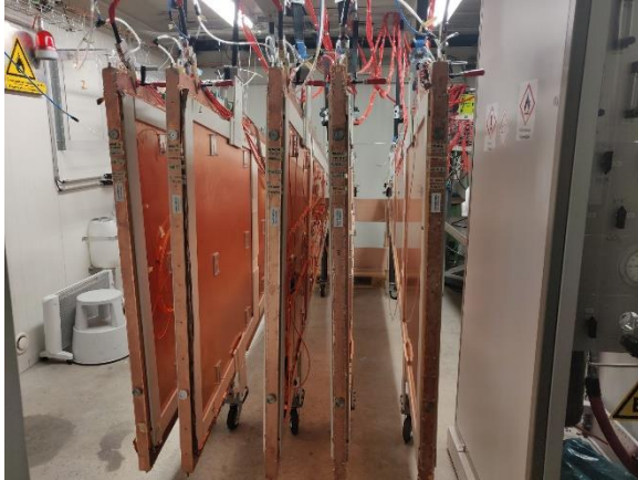
Figure 15. Completed wedges in long-term HV testing [Madhoun, 2019].
