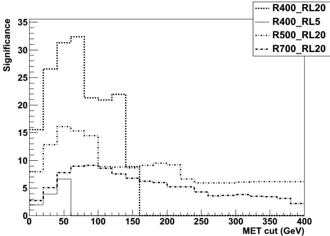
Fig. 4: Plot of significance of cuts made on the MET of trilepton events passing selection with Drell-Yan processes suppressed and Z mass window excluded. For the four points in the mUED parameter space chosen, the highest signal significance is obtained with a cut on the MET excluding events with MET less than about 50 GeV.
