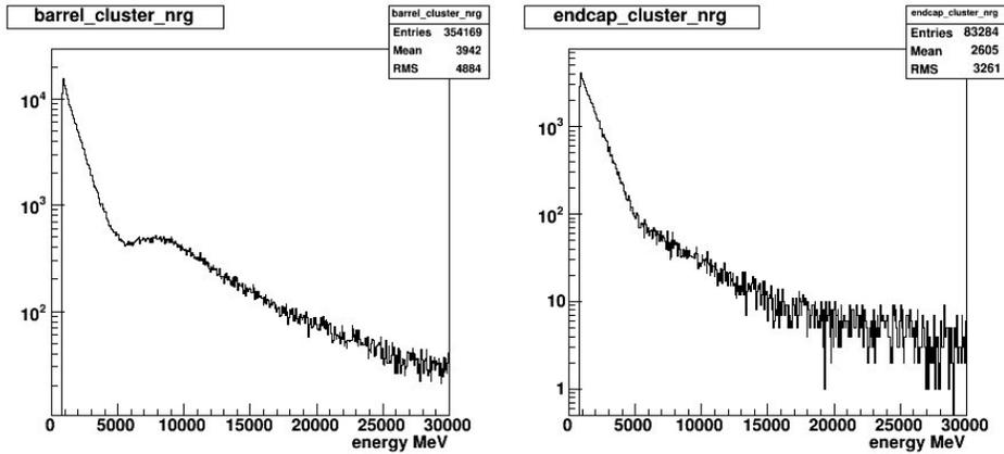
Figure 3: The spectrum of cluster energies in the barrel (left) shows muon energy deposits from around 5 GeV. This structure is not visible for the endcap (right).
