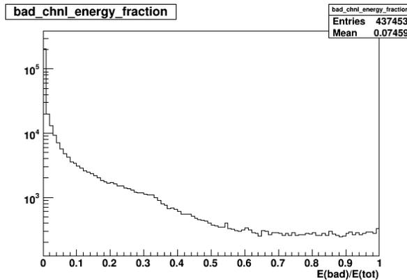
Figure 1: The ratio of the bad channels’ energy to the total cluster energy displays some clusters produced by the presence of bad channels.
