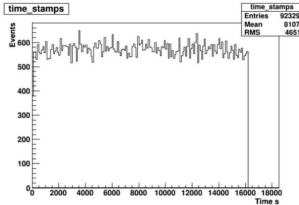
Figure 2: Events are triggered at a constant rate throughout the run.
