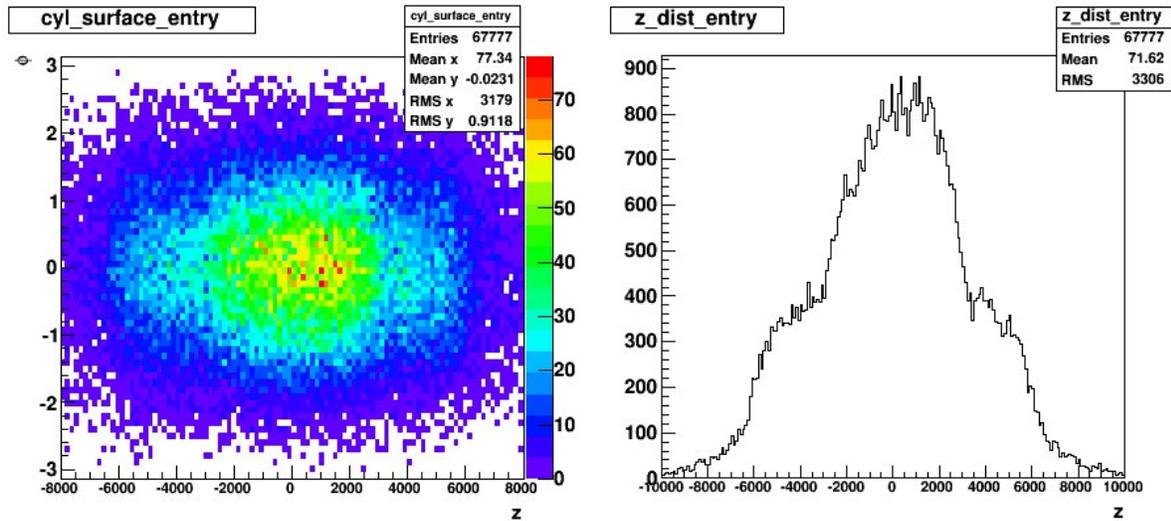
Figure 11: Track entry points on 2 m radius cylinder. Slightly more tracks in positive z explained by the large shaft above the detector.
