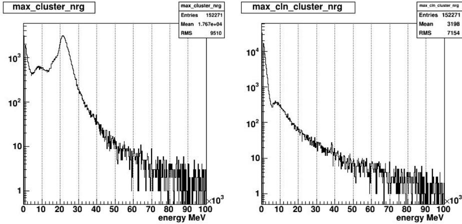
Figure 9: Plotting the spectrum of the maximum cluster energy in each event, and then the same with clean clusters, many spurious processes due to noise are filtered out leaving behind what appears to be the proper spectrum for run 121275.
