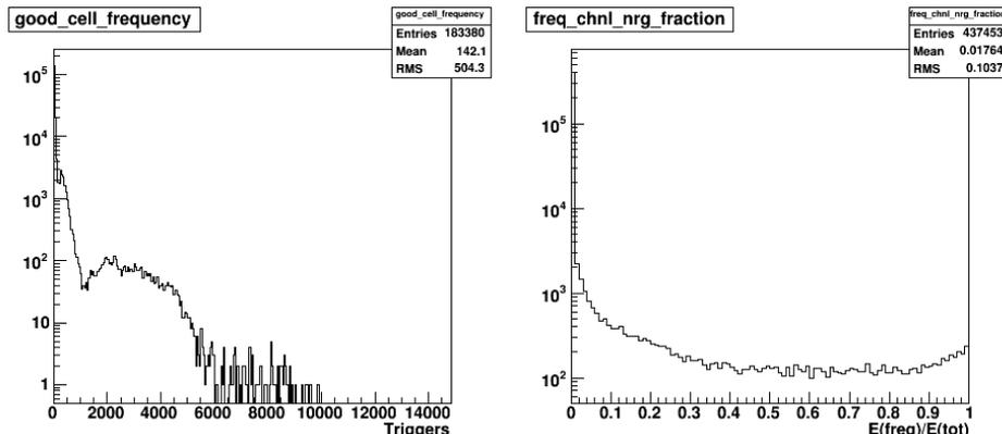
Figure 6: a)Plotting the number of times each channel in the detector is triggered led to choosing to cut channels which trigger more than 6000 times b)Plotting the fraction of each cluster’s energy due to channels which triggered more than 6000 times in the run illustrated that some of these channels are indeed responsible for entire clusters.
