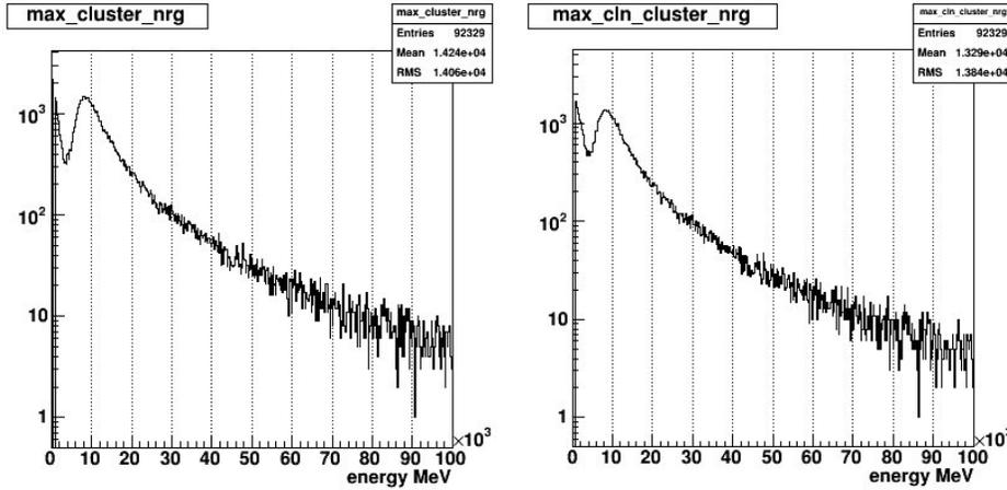
Figure 8: Plotting the spectrum of the maximum cluster energy in each event, and then the same with clean clusters, there is little difference for run 121569.
