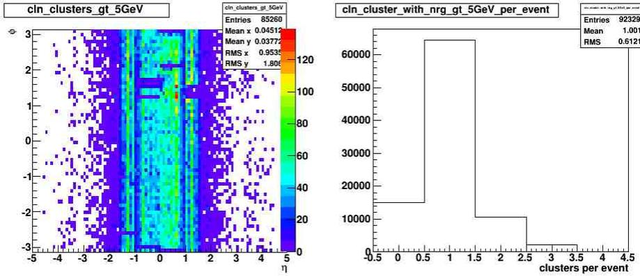
Figure 7: a)The map of maximum clean clusters with energy greater than 5 GeV exhibits a flatter distribution than in figure 5 b)The number of clean clusters with energy greater than 5 GeV per event distributed closely around 1.
