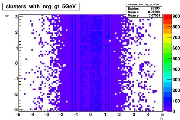
Figure 5: This  $\eta - \phi$  map of the clusters with energy greater than 5 GeV indicates that some cells create frequent clusters.
