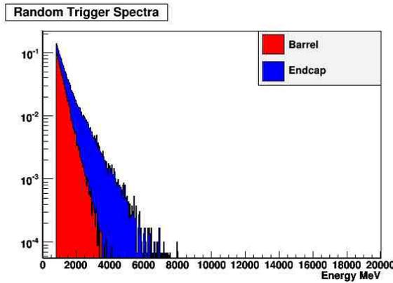
Figure 4: The spectra of cluster energies in the barrel and endcap from randomly triggered events (normalized in this plot) gives us a representation of the noise present during the run.
